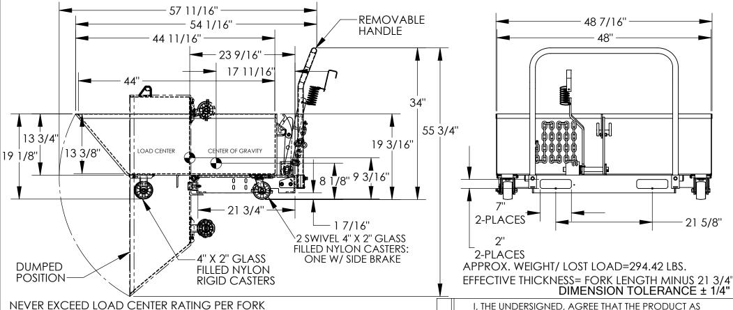
TRUCK MANUFACTURER'S GUIDELINES. DO NOT USE THIS FORK TRUCK ATTACHMENT IF LOAD WILL EXCEED FORK TRUCK MANUFACTURER'S LOAD CENTER RATING.
